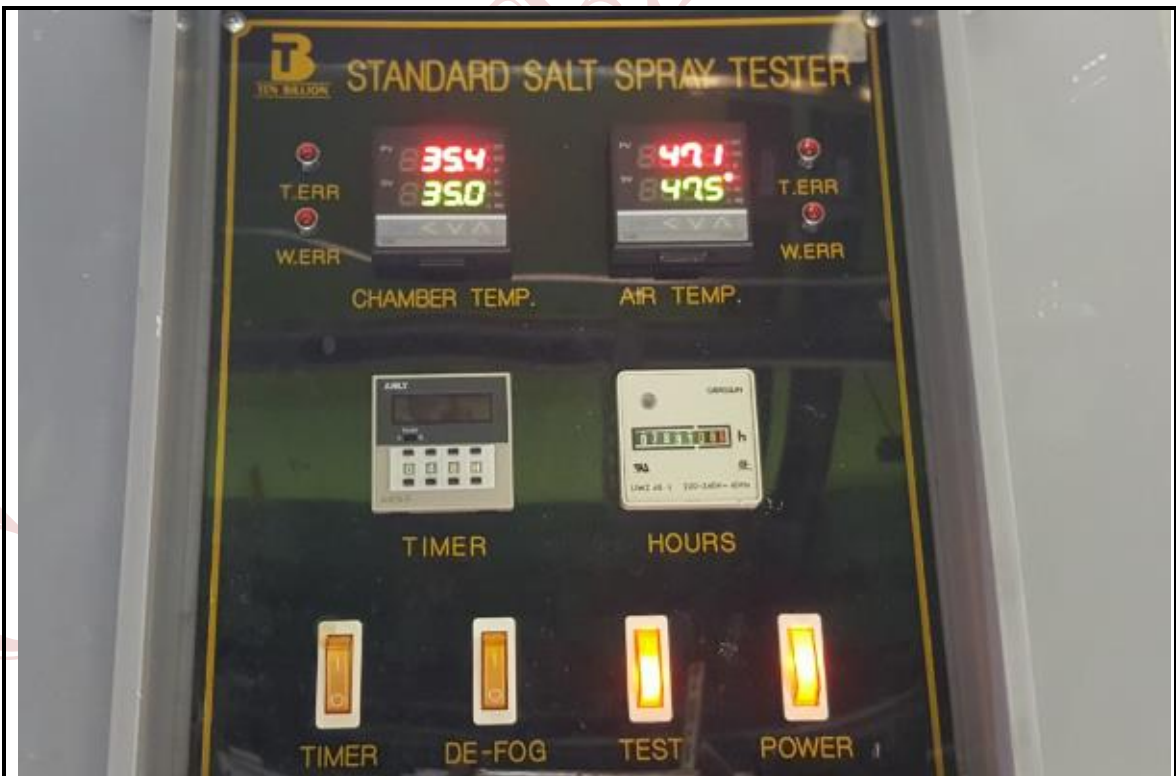
Chamber Setup of Salt Spray Test
